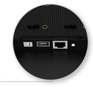
**RS-232 Control** Control, scale and customise your display over long and short distances using RS-232,
