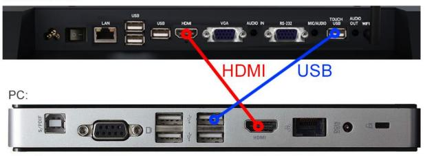
**Figure 4 Screen to PC Connections**
