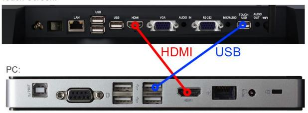
**Figure 1 Screen to PC Connections**
