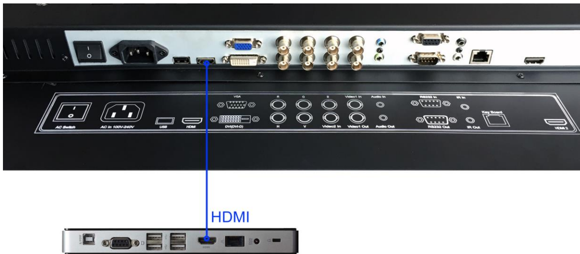
Figure 7 Screen to PC Connections
