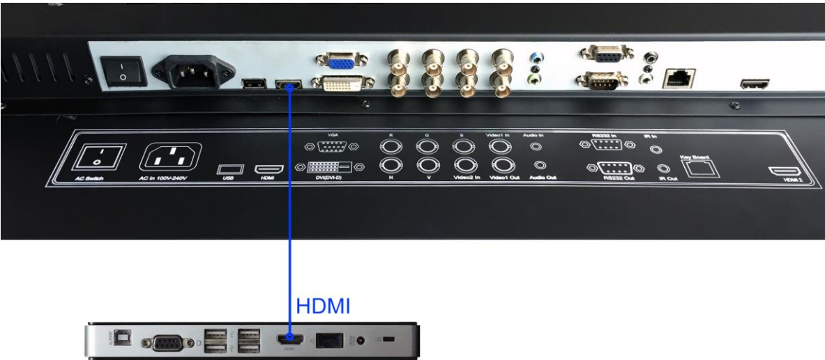
Figure 1 Screen to PC Connections
