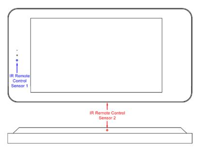
Figure 2 Product Overview - IR Remote Control Sensors
